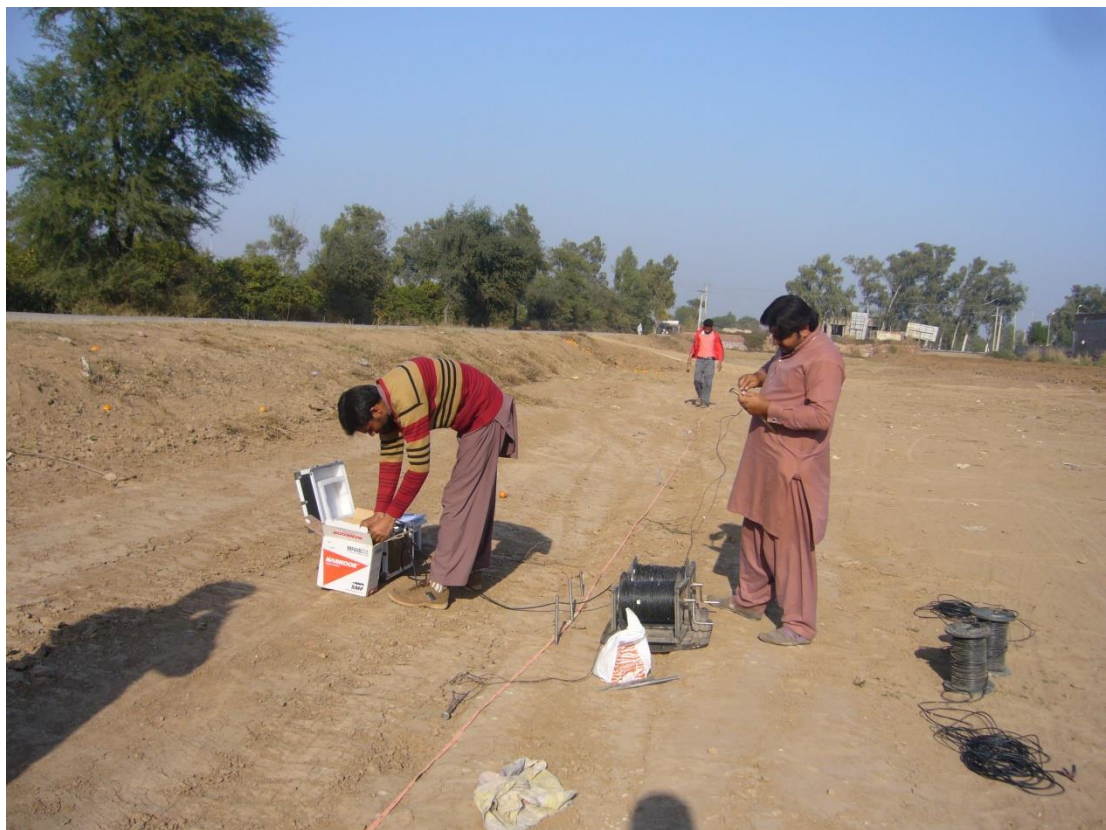
Electrical Resistivity Survey at Shaheen Enclave Housing Scheme, Sargodha
